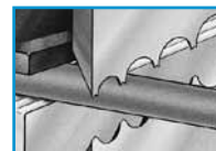
Gripper holds the wire securely in position.
