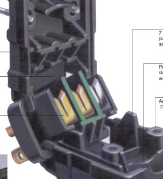
7 load-bearing lugs assure positive fit as the blade holder and sides are closed.
