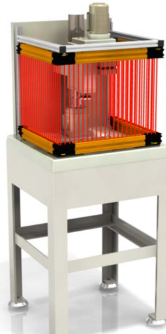
Figure 45. Cascaded light screens guarding a u-shaped cell
