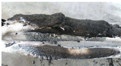
Figure 6: Fire resistant joint before, during and after a fire resistant test
